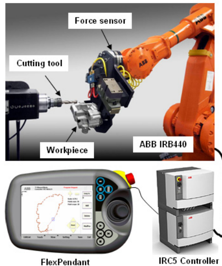
Fig. 1. System setup for robotic machining with force control
