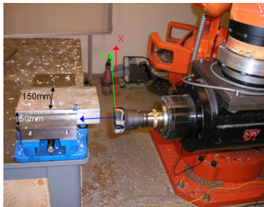
Fig. 6. Robotic end milling process setup
