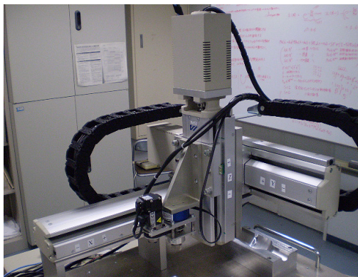
Fig. 2. Developed desktop Cartesian-type robot with abilities of compliant motion and stick-slip motion.
