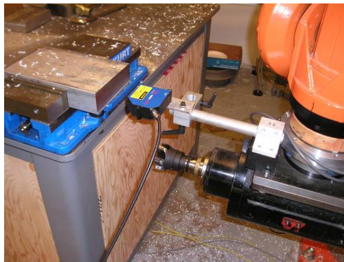
Fig. 16. Setup of aluminum end milling and surface scan
