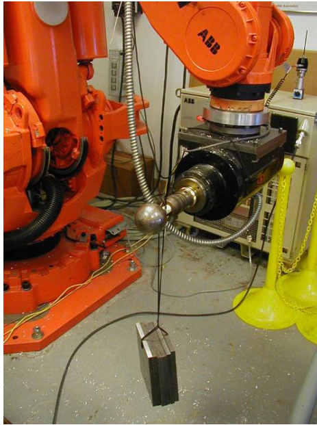
Fig. 14. Methodology of robot stiffness measurement
