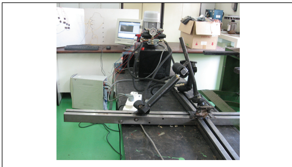
Fig. 2. Fabricated Ball and socket actuator
