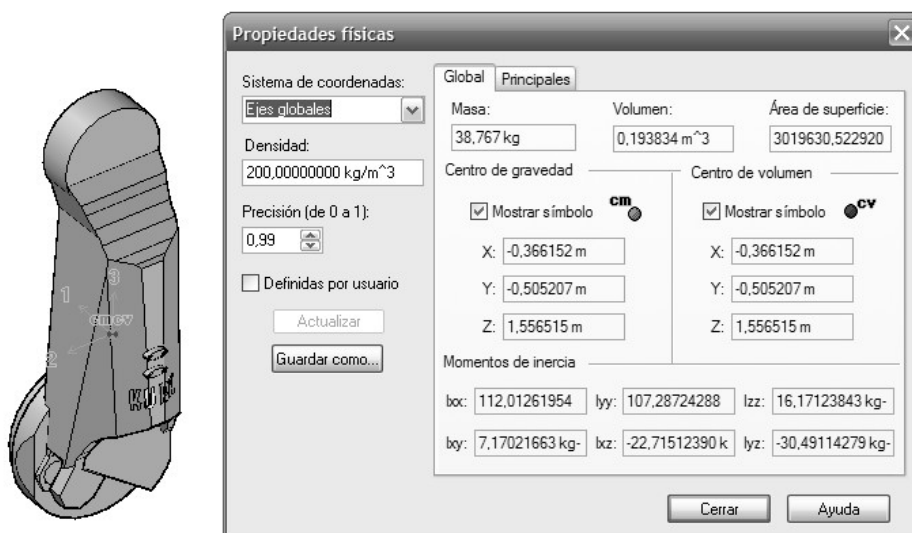
Fig. 8. Inertia obtained in Solid Edge®.
